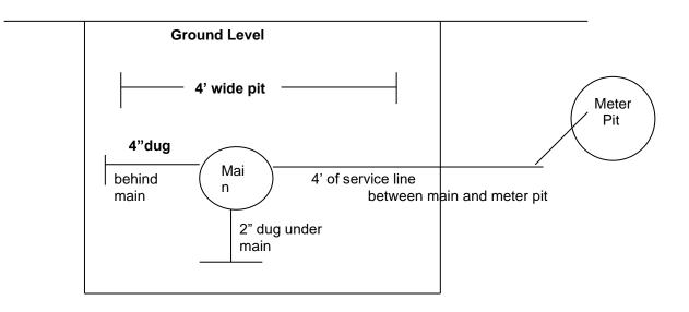
\*\* Tracer Wire (#12 Copper Wire) to be placed from the Main Line to Meter Pit and from the Meter Pit to the Residence. \*\*
