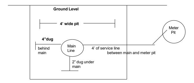
\*\* Tracer Wire (#12 Copper Wire) to be placed from the Main Line to Meter Pit and from the Meter Pit to the Residence.\*\*
